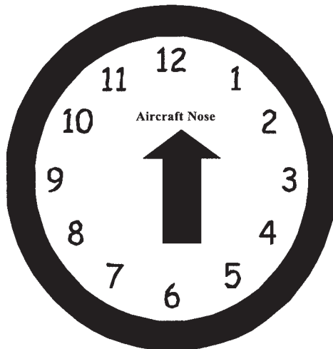
Figure 3–1: Direction Indication Based on Analogue Clock Face
