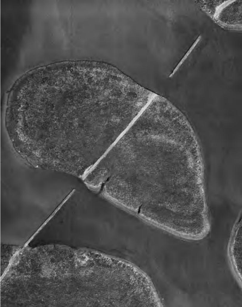
Figure 6–2: Vertical Photograph—Roads Cut by Flooding in Western Australia, March 1999.(RAAF Photograph)
