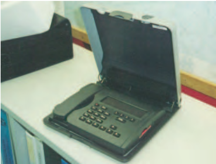
Figure 6–1: Inmarsat M Equipment ( Pacific Emergency Management Associates Pty Ltd )
