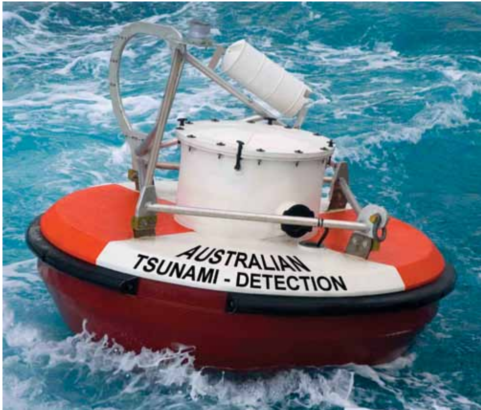
Figure 4.1 The surface component of an operational deep-ocean tsunami detection buoy
