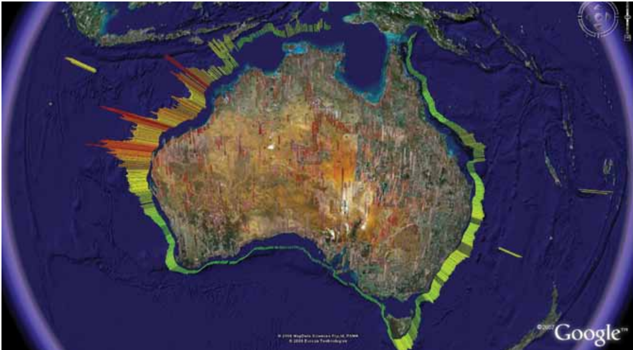
Figure 2.2 An example Australian tsunami hazard map at the 100m water depth contour.
