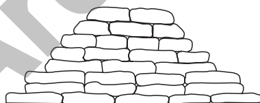
Figure 6:3 Example of sandbag wall construction
