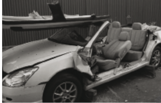
Figure 10:19 Forward Roof Flap
