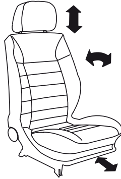
Figure 10:32 Seat movement range
