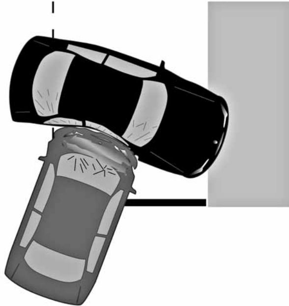
Figure 10:39 Side impacted vehicle on wheels
