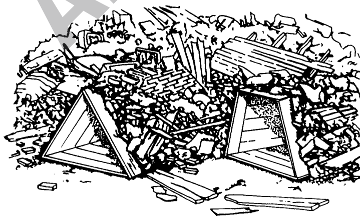
Figure 14:30 Different shapes of tunnels
