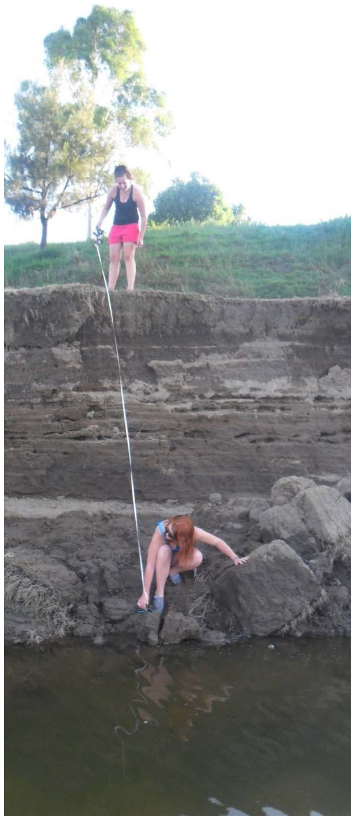
3.9 metres depth of land lost at Harlin (photo courtesy Jenny Moore) Source: Exhibit 41, Statement of Jenny Moore, 7 April 2011 [p13]
