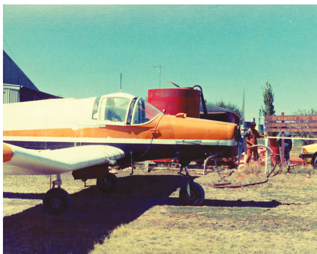
The Benambra firebase in full use a few years later, with a Fletcher F-24 being loaded with retardant.
