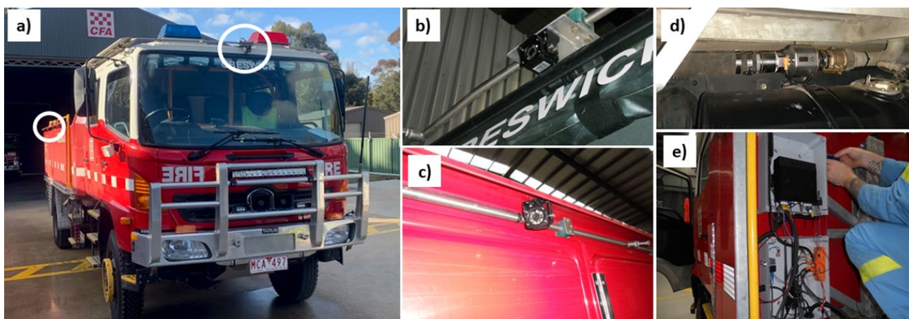
Figure 1: The smart tanker that includes water flow meters and video cameras: a) the circles show the locations of the side and forward mounted cameras, b) the forward-facing camera above the windshield, c) a side (left) mounted forward-facing camera, d) one of the 2 flow meters above the fuel tank and e) weatherproof boxes containing data loggers and modems on the deck behind the left side of the cabin.
