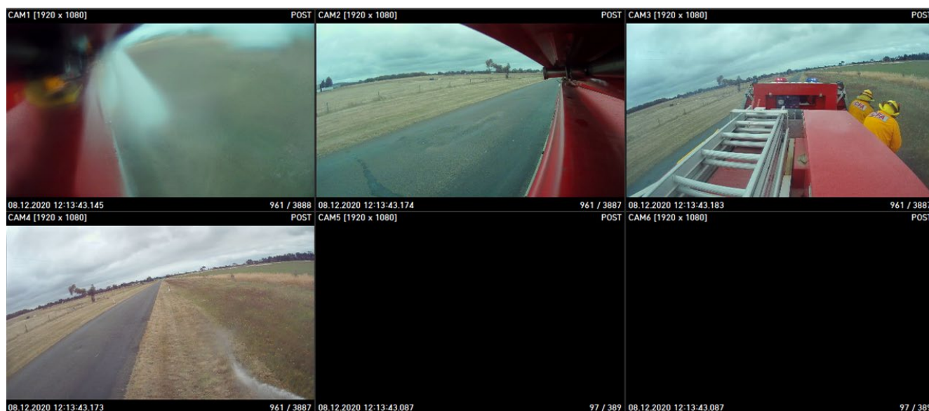
Figure 2: Example screenshot of the view from the 4 cameras installed on the smart tanker: CAM1 rear, right side facing forward (obscured by spray), CAM2 rear left side facing forward, CAM3 rear elevated facing forward showing crew bay and cabin and CAM4 top of cabin facing forwards.
